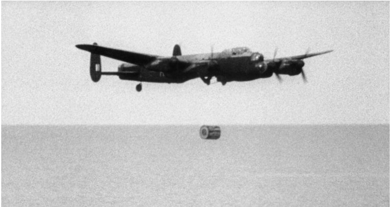
Avro Lancaster with a Bouncing Bomb conducting trials at low level over Reculver Bay, Kent, in April 1943.(IWM)
